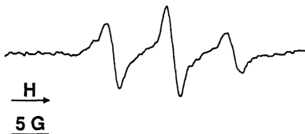
FIGURE 4 ESR spectrum recorded during the reaction of vitamin E, vitamin C and PS with methyl linolenate at 90°C, after hydration of the sample. The spectrometer settings were: microwave power, 20 mW; modulation amplitude, 2 G; receiver gain, 8 \times 10^4 .
